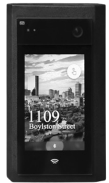
Your mobile device will act as your “key” to the building. Visitors tap the upper-right corner to access the directory.
